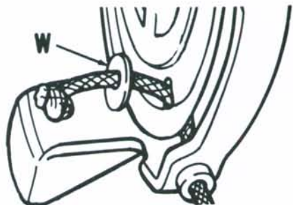
Fig. 11—Install rope on pulley so that washer (W) is between rope knot and pulley.
